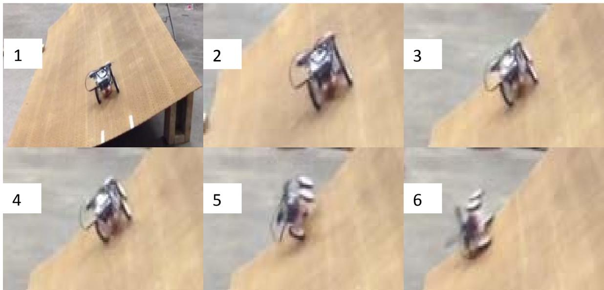
Figure 4. The video frames captured at different times during a rollover test (frame 4: the start of the rollover, frame 5: rolling tractor and frame 6: overturned model tractor).
