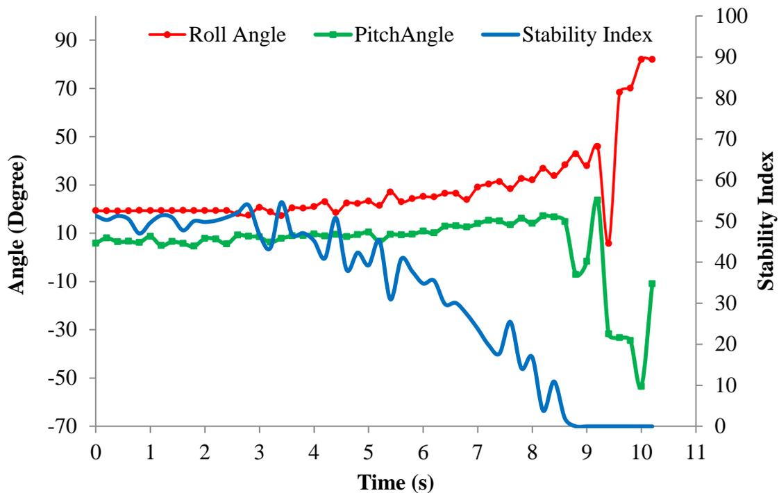
Figure 6. Change of roll angle, pitch angle and roll stability index value with time at a speed of 0.25 m/s.
