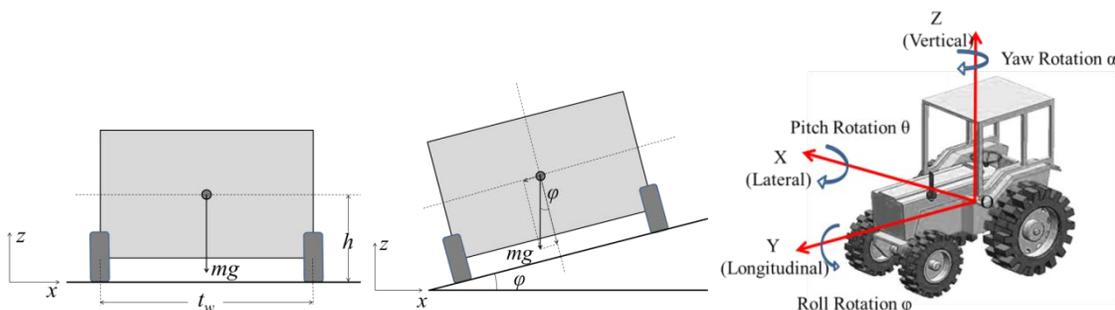
Figure 2. A rigid vehicle model and the roll, pitch and yaw rotations of a tractor.
