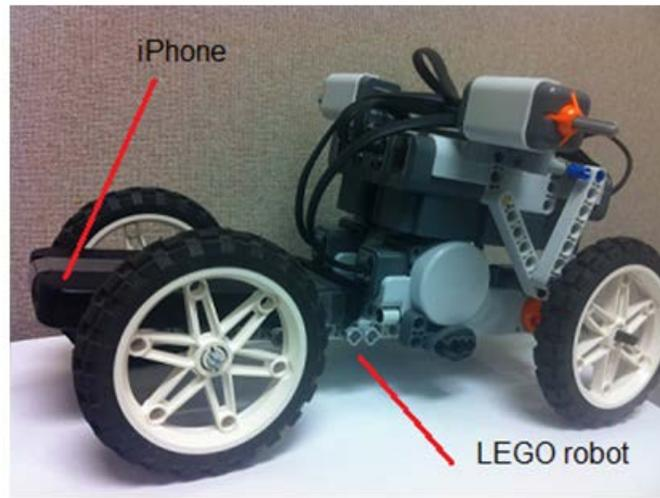
Figure 3. The location of the phone on the model tractor.
