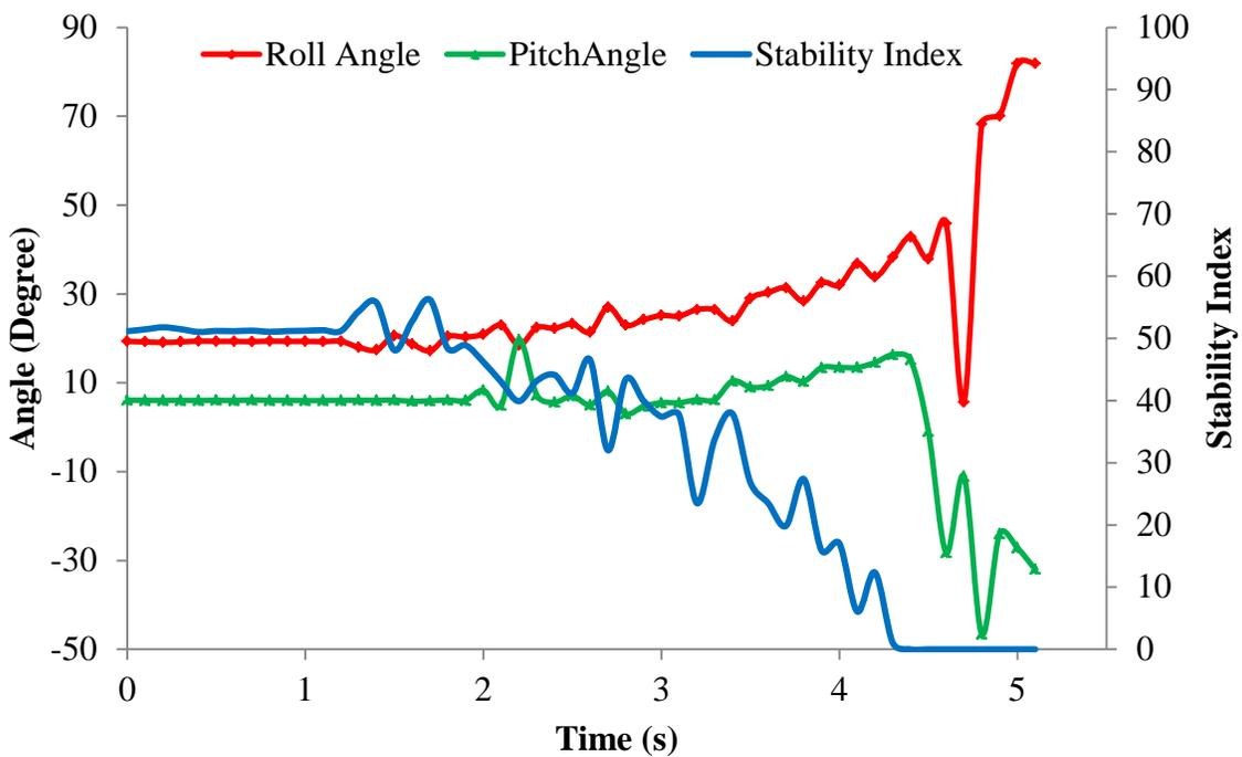
Figure 8. Change in roll angle, pitch angle and roll stability index value with time at a speed of 0.5 m/s.
