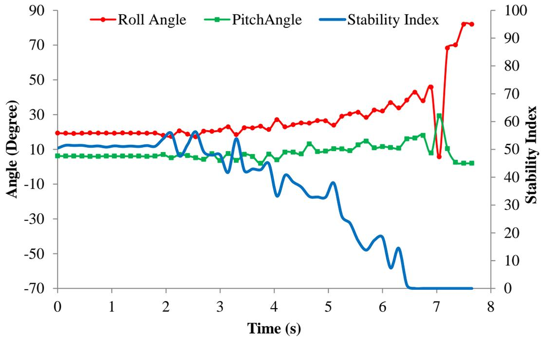
Figure 7. Change in roll angle, pitch angle and roll stability index value with time at a speed of 0.33 m/s.
